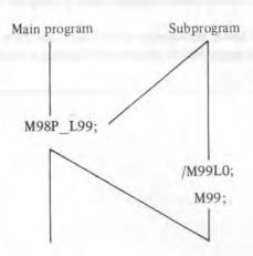
If the optional block skip is turned off in this program, the repetitive count becomes zero and control is passed to the main program when the subprogram end command (M99) is executed.
