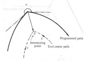
Straight line to straight line in the case in which it goes around at a narrow angle (less than  $1^{\circ}$ ) and the offset vector becames abnormally large.
