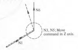
As there are two move command blocks not included in the selected plane and the block N6 cannot be entered into the buffer storage, the tool center path is calculated by the information of N1 in the figure above. That is, in the system 6M, the offset vector is not calculated in start up and the overcutting may result.
