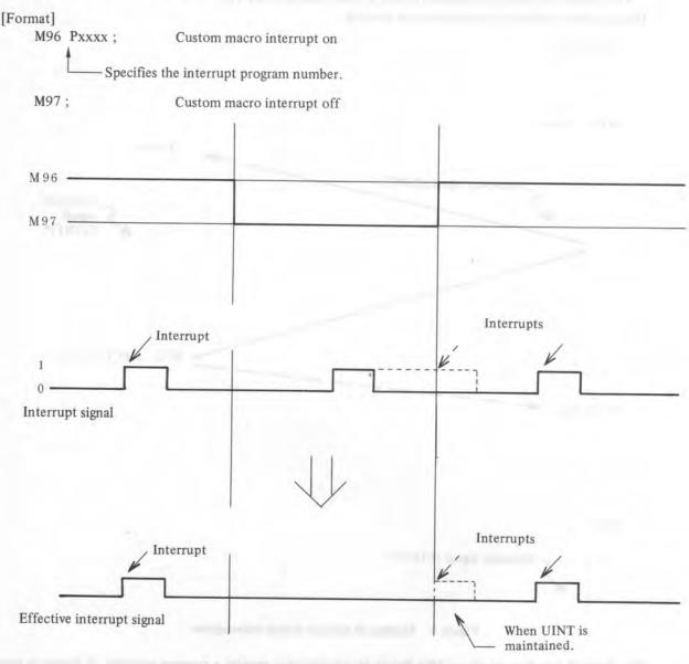
Figure 2.2 Relations between M96, M97, and interrupt signal
