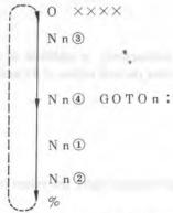
In the above diagram, the execution time increases in the order of (1), (2), (3) and (4). Therefore, it is efficient that GOTO n to be executed frequently be programmed nearer to the Nn block, viewed in the forward direction.
