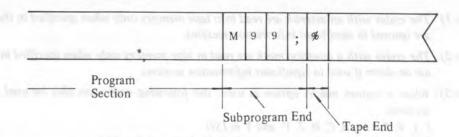
A subprogram must be used after being entered into the tape memory area.
