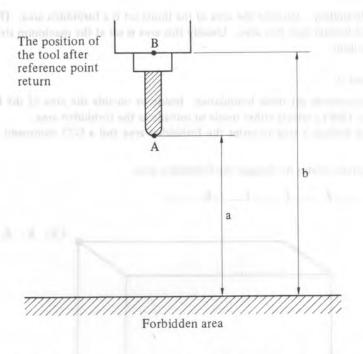
If point A (The top of the tool) is checked, the distance "a" should be set as the data for the stored stroke limit function. If point B (The tool chuck) is checked, the distance "b" must be set.
