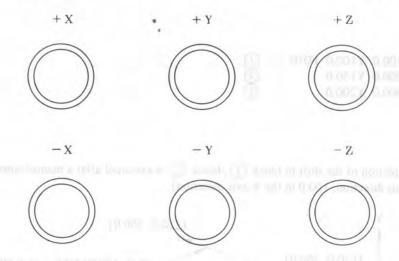
The selected axis is moved for a specified distance by pushing the axis selection switch once.
