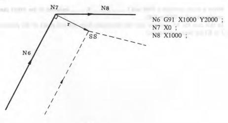
Two blocks without tool movement should not be commanded consecutively. If commanded, a vector whose length is equal to the offset value is produced in a normal direction to tool motion in earlier block, so overcutting may result.
