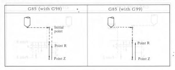
This command is equal to G84 except that the spindle does not reverse at the hole bottom.
