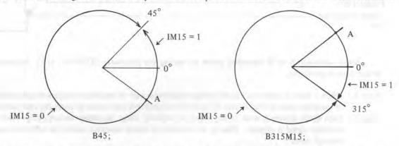
(Note) Although M15 is processed in NC, both the MF and M code are transmitted to the machine side. Therefore, return FIN to NC.
