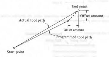
(Note 2) In taper cutting, if usual tool offset is performed, too much or little a depth of cut is generated.
