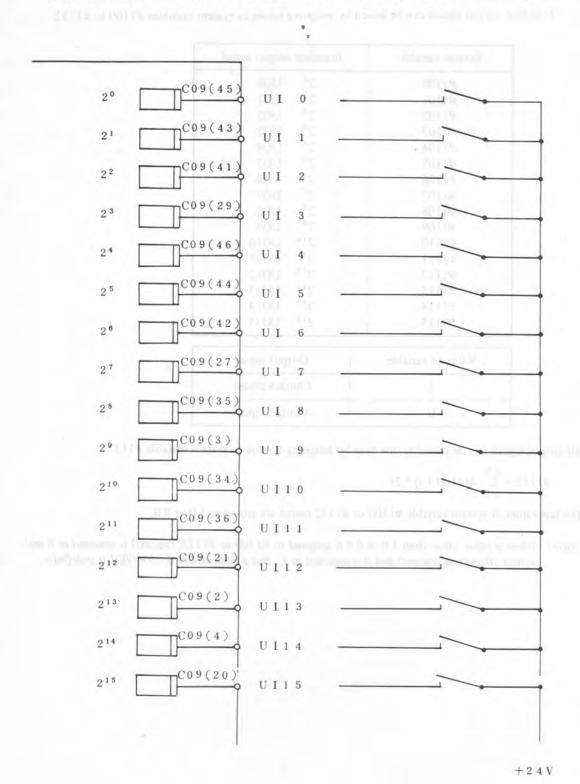
(Note 2) The following diagram shows the connection of input signals for a custom macro.
