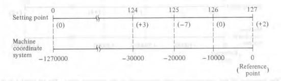
The end of the compensation table corresponds to the reference point and the setting point 126 is at -10000 from the reference point and the other setting points correspond to the position which is shifted -10000 each other.
