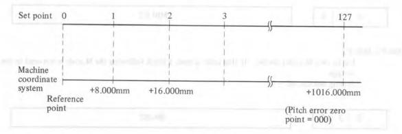
Here, the pitch error compensation interval, which is set by parameter with parameter number  $163 \sim 166$ , is 8000.
