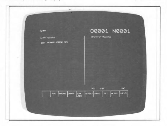
By depressing ALARM software key alarm contents and instructions to an operator are displayed concurrently.
