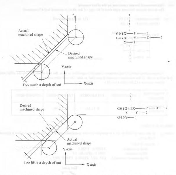
(Note 3) When the offset amount is larger than the move command value, the direction of the actual tool movement becomes opposite to the programmed direction.
