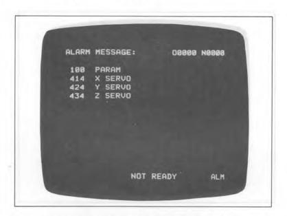
(Note) When an alarm occurs the alarm message is usually automatically displayed.
