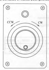
Clockwise rotation . . . . . . + direction Counterclockwise rotation . . . . . . - direction (The direction varies with machine tool builder.)
