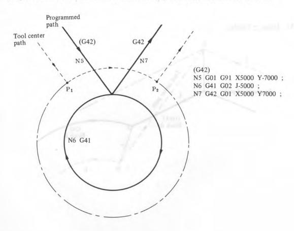
In the above case, the tool center path does not go around a circle but moves only from point P1 to P2 along an arc.
