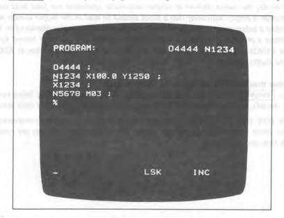
See Section IV 5.16 for which program to display. Pressing a PAGE button displays program contents in sequence. Press the  $^{PAGE}$  button displays the contents in the normal direction; the  $^{PAGE}$  button, in the reverse direction.
