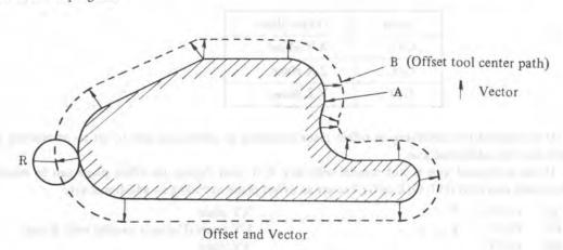
Cutter compensation has two types (B and C). In this section, only type C is explained. The difference between B and C is as follows.
