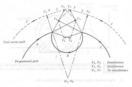
(b) If the interference occurs after correction (a) the tool is stopped by an alarm.
