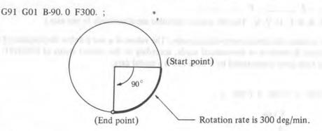
(Note 3) In interpolation including the 4th axis (Rotating axis A, B or C), the unit of the cutting feed (degree) is changed into inch (or mm) and the cutting feed rate in the  $\alpha - \beta$  cartesian coordinate system is controlled so that it is equal to that specified by F code. The feed rate of the rotational axis is calculated as shown in (Note 1) and its unit is changed into deg. per minute.
