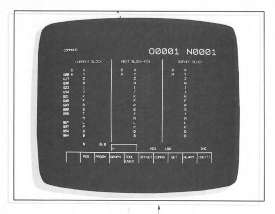
When depressing COMND software key, 9" CRT's three screen display data appears on one screen as shown in the above figure.
