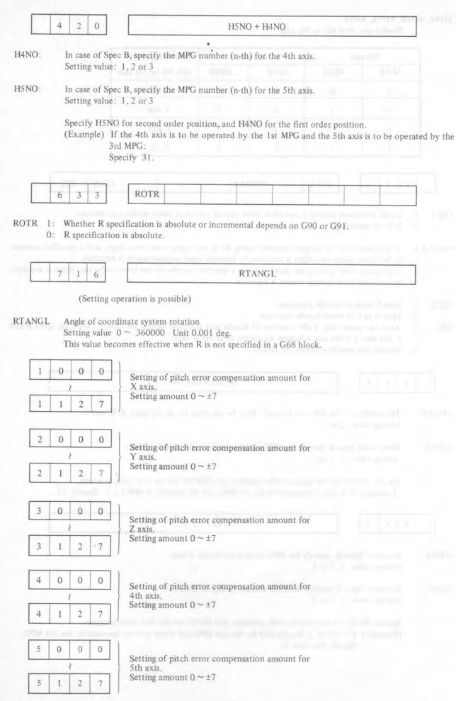
The list of parameters which can be set by the setting operation (address SET) is as follows:
