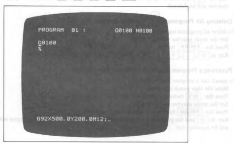
When a keying error occurs, press the CAN key. The character keyed in last will disappear. Keep pressing the CAN key to erase characters one by one from the last. A block of more than 32 characters is too long. Separate the block at an appropriate breakpoint.
