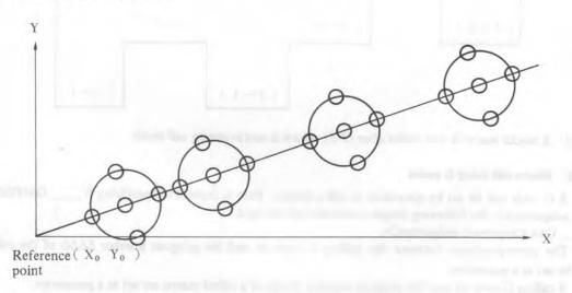
For a drilling work of the pattern, in which a bolt hole circle described in (Example 10. 7. 2) is overlapped on an unequal spacing line at angle described in (Example 10. 7. 3), a program must be made by using macro and canned cycles as follows.
