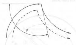
When  $\theta \le \theta p$ , the corner is regarded as inside.  $\theta p$  value is set by parameter (No. 335) ( $1 \le \theta p \le 179$  unit°) If  $\theta$  is almost equal to  $\theta p$ , the decision may include an error within 0.001°.
