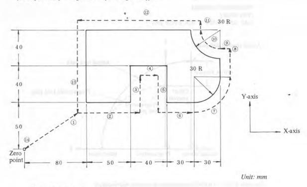
Tool diameter 20 mm dia. Offset number 01 Offset amount +10.0 mm
