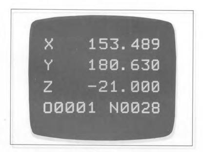
The relative position is displayed in which the position reset by an operator is zero.
