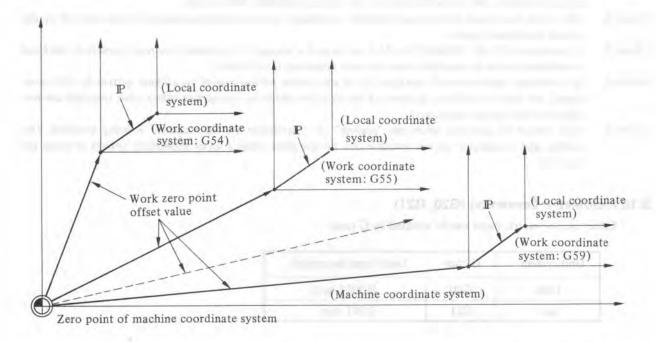
When a local coordinate system is set, the move commands specified in the absolute mode (G90), which are subsequently specified, are the coordinate values in the local coordinate system.
