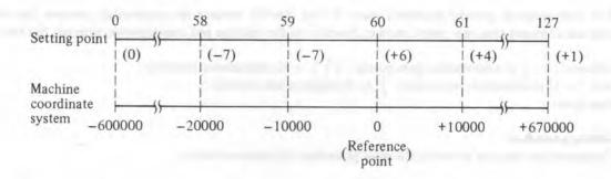
The setting point 60 corresponds to the reference point. The setting point 61 is at +10000 position and the other setting points corresponds to the position which is shifted +10000 each other.
