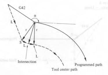
The intersection in the above figure is the intersecting point between offset paths by r distance of two blocks.
