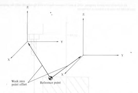
Work coordinate systems 1 to 6 are established after reference point return after the power is turned on. When the power is turned on, G54 coordinate system is selected.
