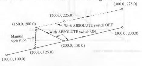
(d) When the command following manual operation is one axis command, only the commanded axis returns to the programmed absolute position of the axis.
