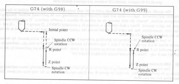
This command specifies the spindle to rotate clockwise at the hole bottom, and then a left-handed tapping cycle to be performed.
