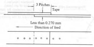
(c) Make sure the punched holes of the overlapped tape sections at the joint are correctly aligned. Use special care with the feed holes.
