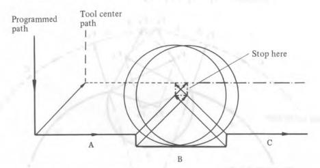
Although the interference does not actually occur, the tool is stopped by alarm (No. 41) because the direction of the tool path after cutter compensation is different from that of the programmed path.
