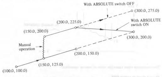
(c) The FEED HOLD button is pushed during the execution of block (2), and a resetting action is taken, after a manual operation process (Y + 75.0), and then the block (2) is input again.
