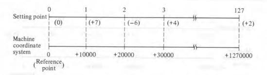
The beginning of the compensation table corresponds to the reference point. The set point 1 is at +10000 position and the other setting points correspond to the positions on the machine coordinate system which is shifted +10000 each other. Therefore, setting point 128 is at +1270000.
