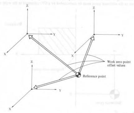
In the use of these work coordinate systems, G92 need not set coordinate systems. Simultaneous use of G54 to G59 and G92 displaces coordinate systems by G54 to G59, so usually they are not used simultaneously.
