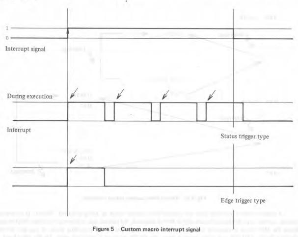
The status trigger type executes the custom macro interrupt when the signal is on; the edge trigger type executes it when the signal turns on. Therefore, the example above shows that four interrupts are executed in the former type; only one in the latter type.
