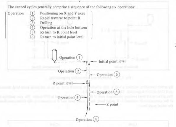
Fig. 7.2.1 Canned cycle operation
