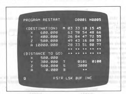
DESTINATION displays the position from which machining is restarted.
