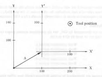
When the tool is positioned at (200, 160) in a G54 state, G92X100Y100; provides work coordinate system 1(X' - Y') displaced by vector A. At the same time all the other work coordinate systems are also displaced by vector A.
