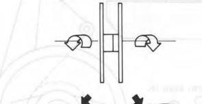
(i) The reel can be dismantled by twisting the reel hub in the direction of the arrow.
