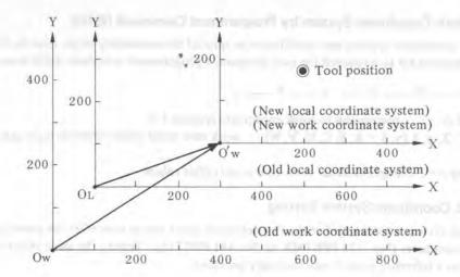
If G92X200.0Y150.0; is specified when the zero point of the local coordinate system is positioned at (100, 150) in the work coordinate system and the tool is positioned at (500, 250) in the local coordinate system, zero point Ow of the work coordinate system and zero point  $O_L$  of the local coordinate system shift to the O'w position.
