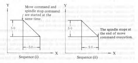
The selection of either sequence depends on the machine tool builder's specifications. In certain cases, these sequences may be provided together in an NC machine. Refer to the manual issued by the machine tool builder for details.
