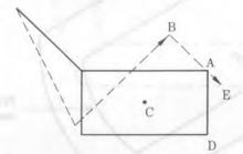
When Reset is effected at point B and then point D is specified, the tool moves to point E regardless of the absolute/incremental command for the movement from point A to point D.
