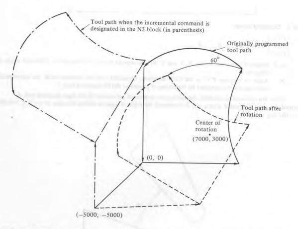
(Note 2) When the first position command block appearing after the G68 block contains an absolute command, both axes on the coordinate system rotation plane must be designated.
