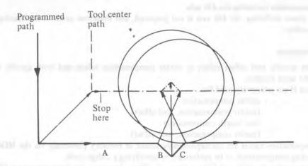
The direction of the tool path is different from that of the programmed path the same as example (a).
