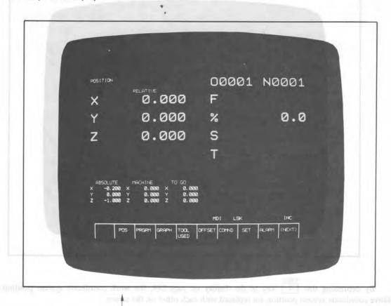
By depressing software key POS , the present position in the relative coordinate system is displayed on the CRT. The present positions and residual move amounts in the work coordinate system and machine coordinate system are displayed at the lower part of the CRT.
