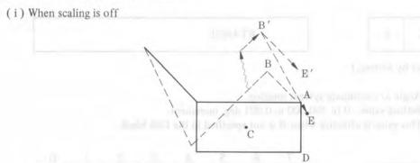
When the command of point D is absolute and both X and Y axes are specified, the tool moves to point E. When the command of point D is incremental, the tool moves to point E'.
