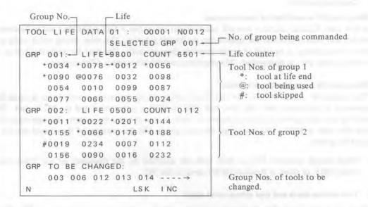
One page displays data on two groups. Pressing the button successively displays data on the following groups. Up to five group Nos., for which the Tool Change signal is being issued, are displayed at the bottom of each page. An arrow shown in the figure is displayed for six or more groups, if any. To know data on a particular group, select address N, input the group No., and press the INPUT button. Pressing the button moves the cursor to GRP of the next group and displays its data.
