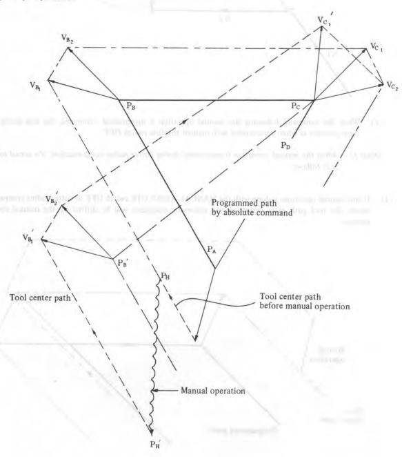
In the above programmed path  $(P_A \rightarrow P_B \rightarrow P_C \rightarrow P_D)$ , suppose that the tool is translated from  $P_H$  between  $P_A$  and  $P_B$  to  $P_{H'}$  by manual operation (after pushing the feed hold button).
