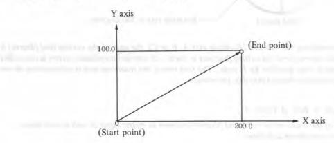
The feed rate commanded by the F code is measured along the tool path. If it is not commanded, the feed rate is regarded as zero.
