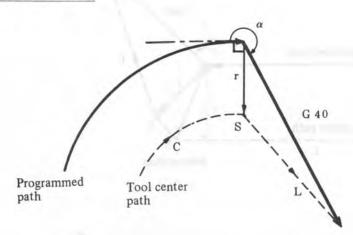
(b) When going around an outside corner at an obtuse angle (90°  $\leq \alpha < 180^{\circ}$ )
