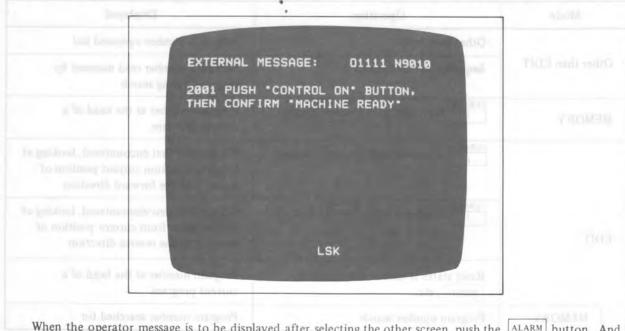
When the operator message is to be displayed after selecting the other screen, push the ALARM button. And when the alarm message is displayed, press the ALARM button again.
