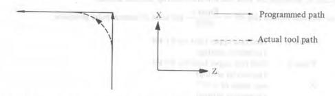
In circular interpolation, the actual arc radius is smaller than that of the programmed arc. (See the appendix.) This error can be minimized by making the acceleration/deceleration time constant of feedrate small.
