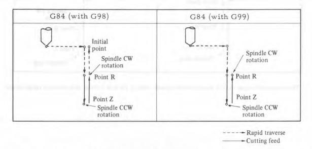
This command specifies that the spindle rotates in the counterclockwise direction at the hole bottom, and a tapping cycle is performed.
