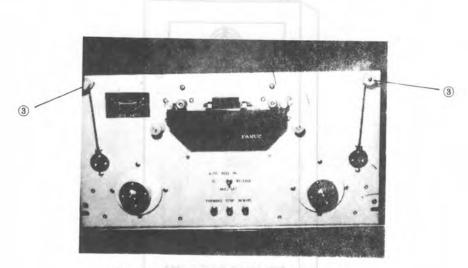
Fig. 1.2 (c) Tape reader with reels front view
