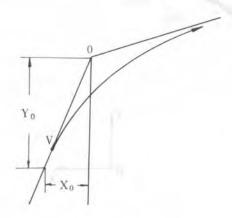
Coordinate values of Xo and Yo in the figure are determined by the feed rate and the time constant of the positioning system using the DC servo motor.
