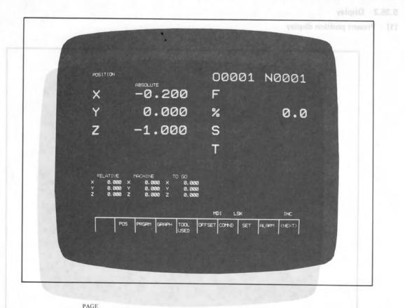
By depressing the weight by key in the display on page 289, the work coordinate system position and the relative coordinate system position are replaced with each other on the screen.
