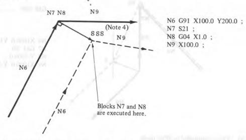
(Note 4) SSS means that tool stops three times by single block operation.
