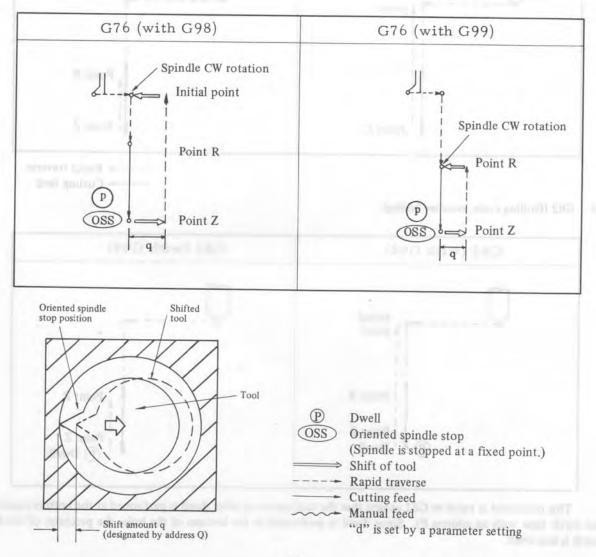
(Note 1) G76 can be used only when the parameter (FIX2) is set to output M codes as the output signals for spindle CCW rotation, spindle CCW rotation and oriented spindle stop.
