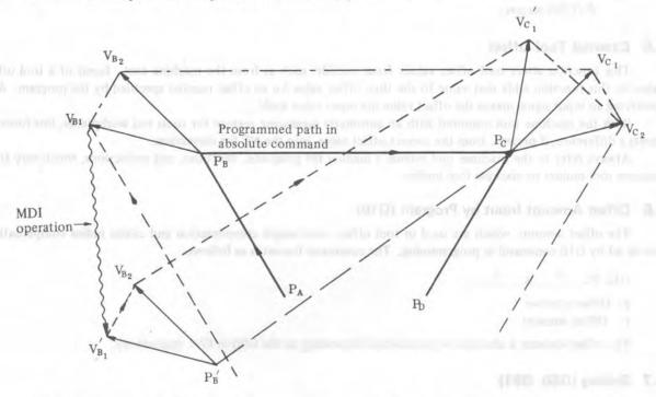
When points  $P_A$ ,  $P_B$  and  $P_C$  are programmed in an absolute command, the tool is stopped by the single block function after executing the block from  $P_A$  to  $P_B$  and the tool is moved by MDI operation. Vectors  $V_{B1}$  and  $V_{B2}$  are translated to  $V'_{B1}$ , and  $V'_{B2}$  and offset vectors are recalculated for the vectors  $V_{C1}$  and  $V_{C2}$  between block  $P_B$ - $P_C$  and  $P_C$ - $P_D$ .
