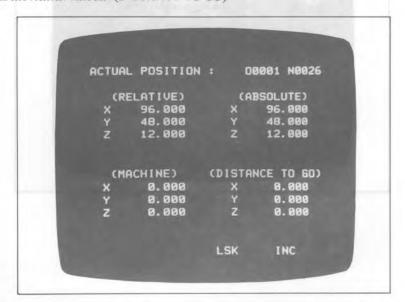
The residual movement amount indicates the movement amount remaining in one block of a command. When the overall display is on, the position of a paticular coordinate system cannot be reset.
