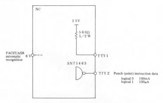
(Note) The +6V for FACIT/ASR automatic recognition must be open when the ASR 33 is used.
