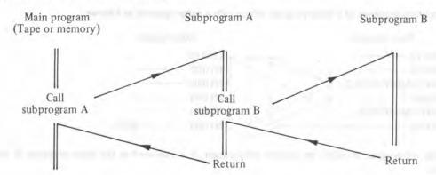
A call command can be used to call a subprogram repeatedly. A call command can specify up to 9999 repeations of a subprogram.
