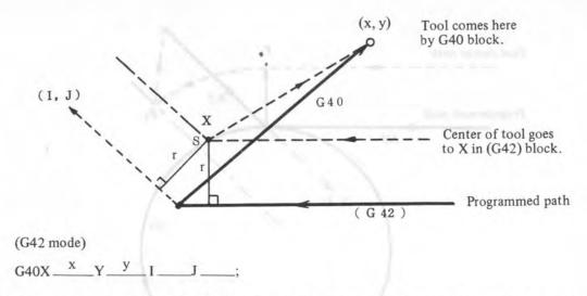
(Note 5) In this case, note that the NC obtains an intersection of the tool path irrespective of whether inner or outer wall machining is specified.
