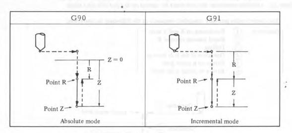
Fig. 7.2.2 Absolute and incremental programming
