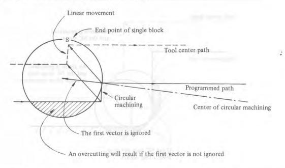
(iv) The start up and the movement in Z axis on the cutter compensation C
