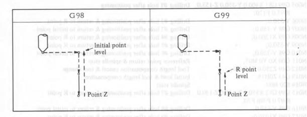
Fig. 7.3 Initial point level and R point level
