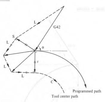
(Note) In the case of type B, when the tool goes around the outside linear  $\rightarrow$  linear at an acute angle less than 1 degree, compensation is performed as follows.
