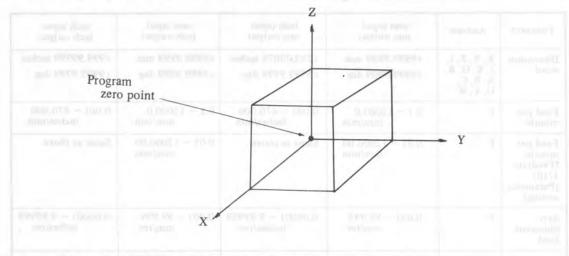
This coordinate system is called the work coordinate system.
