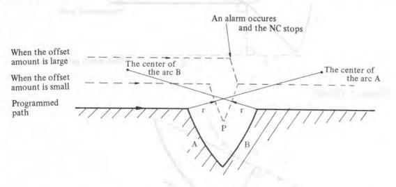
When the offset amount is large as in the figure above, the intersecting point as that in the small offset amount (point P) is not present.
