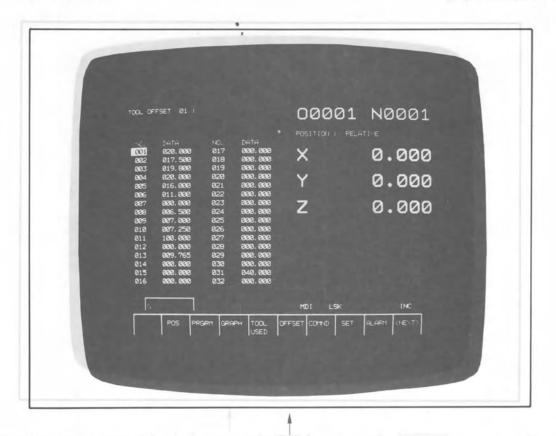
Offset values corresponding to each tool number are displayed by depressing OFSET software key.
