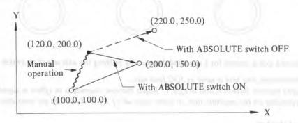
(b) The FEED HOLD button is pushed during the execution of block (2), and the CYCLE START button is again pushed to release the hold state after a manual operation process (Y + 75.0).
