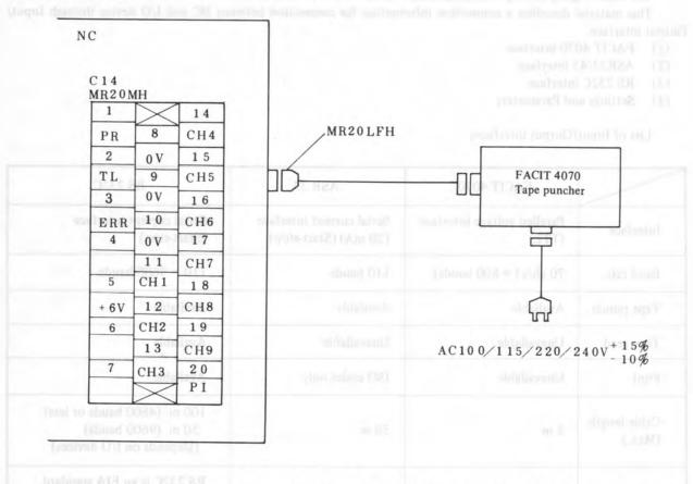
(Note) The input/output interface option does not include the connecting cable running between the FACIT 4070 and NC.
