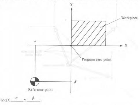
(Note 1) In use of work coordinate system by G54 to G59, G92 command is unnecessary.
