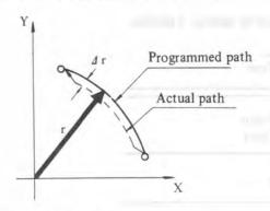
Δr: Maximum error in radius direction (mm)
