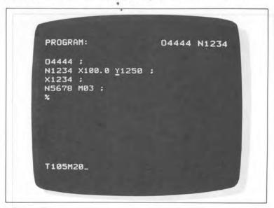
Data cannot be keyed in when a picture displayed by pressing the POS or ALARM button is displayed. If D/H button is pressed twice, address H is selected.
