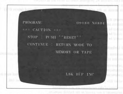
(4) After registering or editing programs 0900 to 09899, call out a different program and effect locking. Locking, while programs 09000 to 09899 are displayed, provides the screen with the figure above in the edit mode. Applying reset displays the program.
