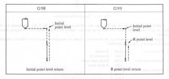
Fig. 7.2.3 Initial point level and R point level
