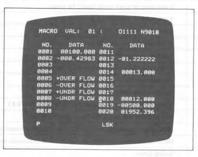
When a variable value is (vacant) (see Section III 14.2.3), a blank is displayed. When an absolute value exceeds 99999999, OVER FLOW is displayed. When an absolute value is not 0 and under 0.0000001, UNDER FLOW is displayed.
