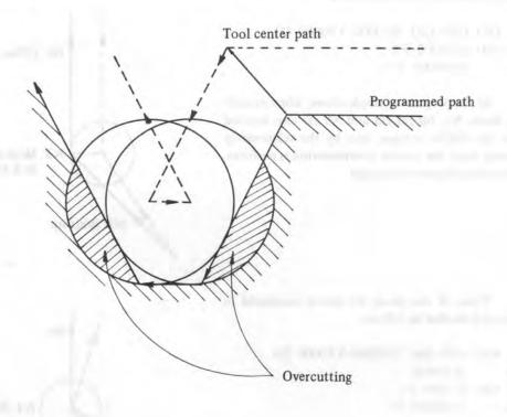
(iii) When machining a step smaller than the tool radius
