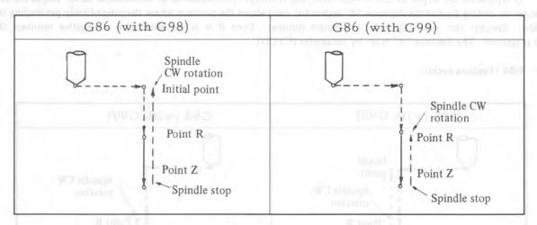
This command is equal to G81 except that the spindle stops at the hole bottom, and returns in rapid traverse.
