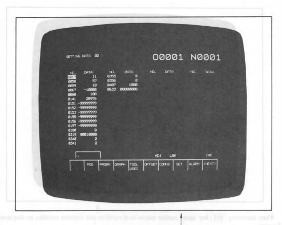
Various setting data are displayed by depressing  $\[ \]$  software key. Running time is also displayed at setting 01.
