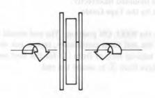
(iv) Twist the reel hub in the direction of the arrows, until the hubs are secured.
