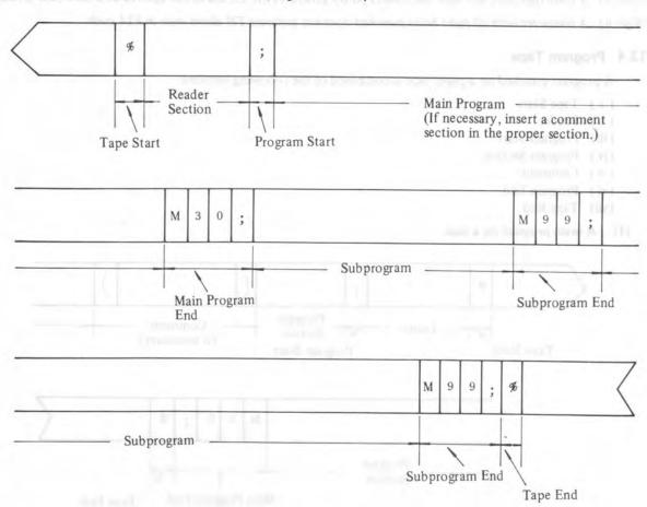
A program including subprograms on a tape must be used after being entered into the tape memory area.
