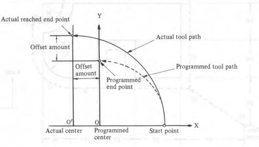
(Example 6.2.2) Cutter compensation in circular interpolation
