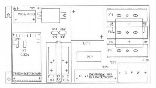
Fig. 2.1 (b) Input unit for control unit and servo unit
