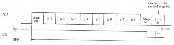
In order to stop data transfer from NC, the CS signal must be switched from ON to OFF within this range.
