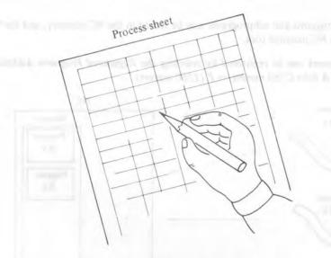
The program on this process sheet is punched on paper tape using a paper tape punch. This paper tape is called an NC tape and is input to the NC.
