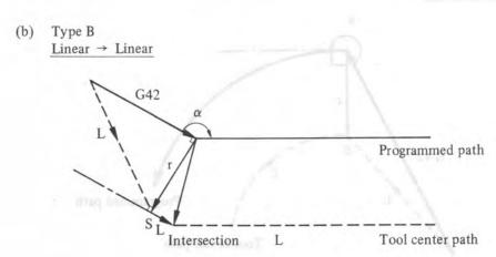
The intersection is the point where two offset paths calculated by continuous two blocks are intersected.
