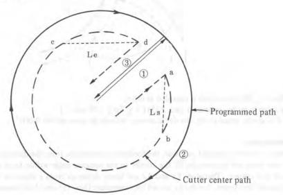
Regarding program (2) of an arc, the feedrate is overridden from point a to point b and from point c to point d.
