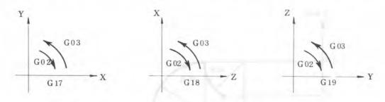
The end point of an arc is specified by the address X, Y or Z, and is expressed in an Absolute or Incremental value according to G90 or G91, respectively. In incremental expression, the coordinate of the end point is specified as seen from the start point of the arc.
