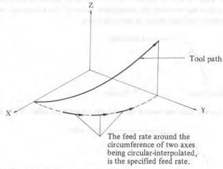
(Note 1) Cutter compensation is effected only for a circular arc.
