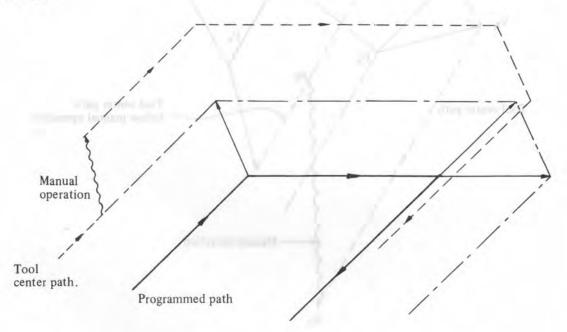
(2) If the manual operation is performed with the MANUAL ABSOLUTE switch ON in the cutter radius compensation C mode, the tool path after restarting the automatic operation by absolute command is as follows:
