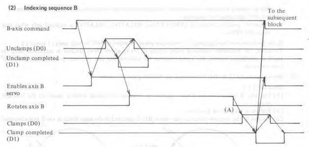
Select sequence A or B described above by setting the parameter (IDXB-No. 315). In-position check is always done at point (A).
