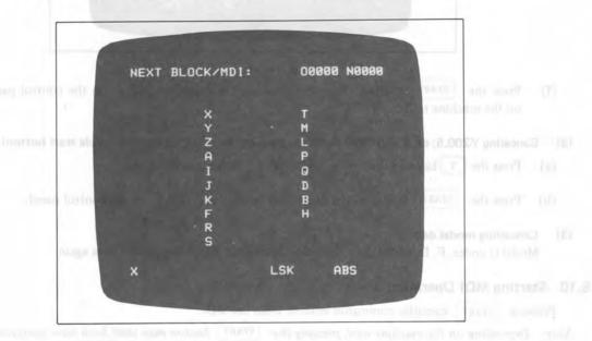
(d) Press the X, 1, 0, ..., 5 keys and the INPUT button in this order. If you are aware of an error in the keyed-in number before pressing the INPUT button, press the CAN button and key in the correct number again. If you notice an error after the INPUT button is pressed, key in the number again from the beginning.
