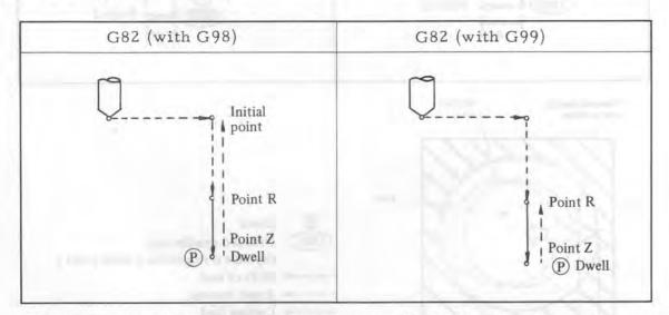
This command is equal to G81 except that the tool moves up after dwell is performed at the bottom (specifies the dwell time with an address P). Since dwell is performed at the bottom of the hole, the precision of the hole depth is improved.
