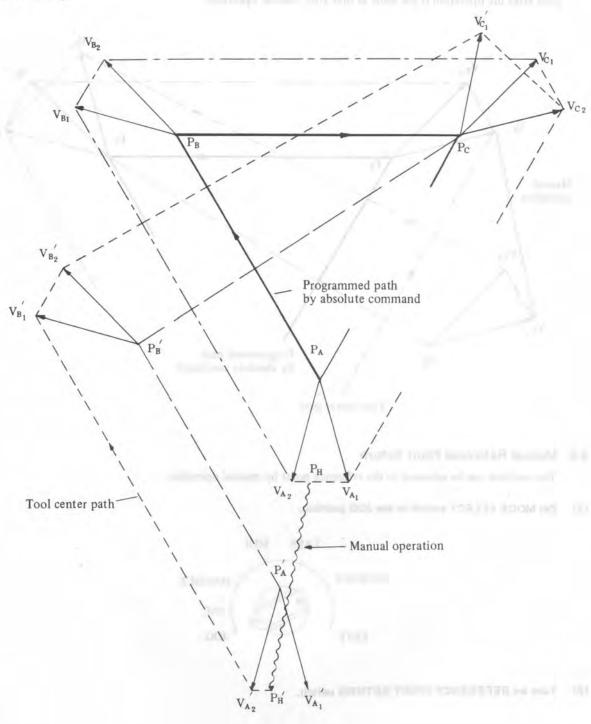
In cutter radius compensation, if during corner machining the manual operation is performed, the tool path after that is determined in the same way as example 1.
