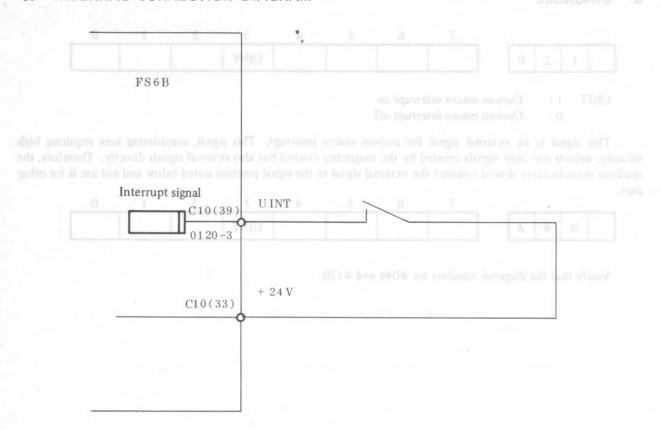
To connect this signal, connection unit 2 is required.
