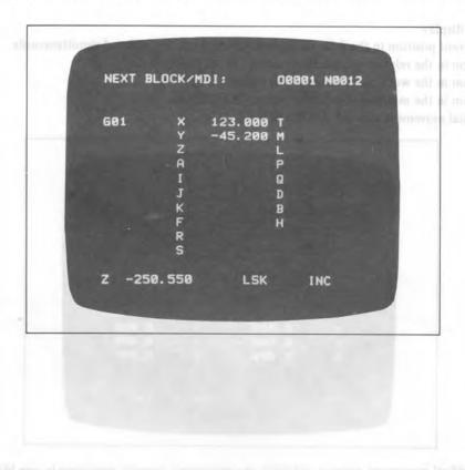
(iii) The command to be executed next but one is displayed in the offset mode by cutter compensation.
