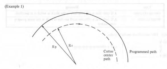
However, if Rc is very small as compared with Rp, Rc/Rp = 0, causing the cutter to stop. Accordingly, the minimum reduction ratio (MDR) is set to set the actual feedrate to F  $\times$  (MDR) when Rc/Rp  $\leq$  MDR.
