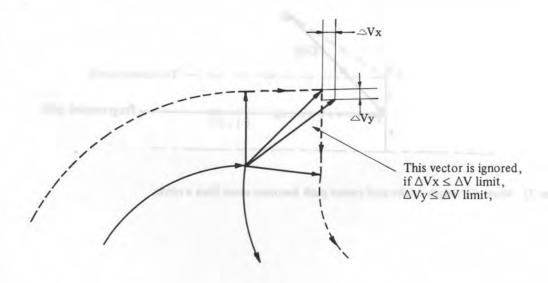
If  $\triangle Vx < \triangle V_{limit}$  and  $\triangle Vy < \triangle V_{limit}$ , the latter vector is ignored. The  $\triangle V_{limit}$  is set in advance by parameter (CRCDL).
