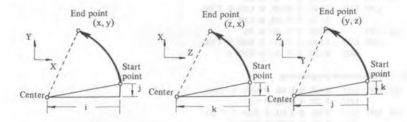
The circular interpolation can be commanded with address R instead of address I, J or K. The command format is as follows.
