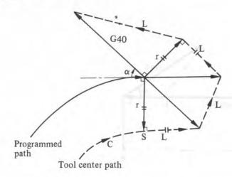
(Note) In the case of type B, when the tool goes around the outside linear  $\rightarrow$  linear at an acute angle less than 1 degree, compensation is performed as follows.
