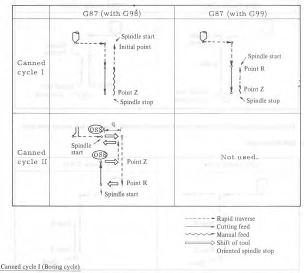
When the tool reaches the hole bottom and the spindle stops, the control goes into the feed hold condition, and the tool can be moved in a manual mode while in this condition. Any manual operation can be performed, but the tool should be drawn out of the hole for safety.
