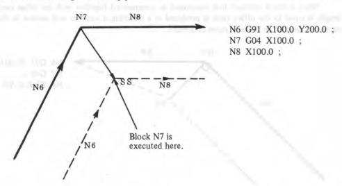
However, when the move distance is zero, even if the block is commanded singly, tool motion becomes the same as that when more than one block of without tool movement are commanded, which will be described subsequently.
