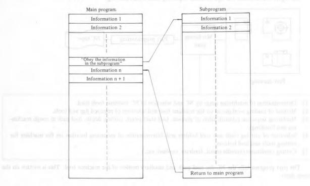
A total of 95 main programs and subprograms may be stored in the NC memory, and the NC uses one of these main programs to move the NC machine tool.
