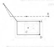
If reset is made at point B, point A in program coordinates is regarded as being present at point B. When the move command to point D is executed, the following movement occurs according to whether the command is incremental or absolute.
