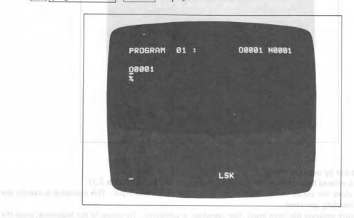
(d) Key in one block according to the process sheet.
