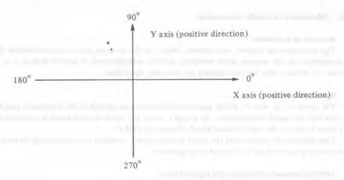
Angle 0 is X-axis positive direction; angle 90° is Y axis positive direction as shown in the figure.
