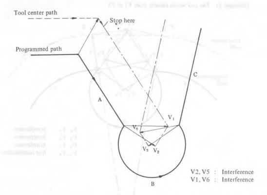
After ignoring the vector V2 and V5 because of interference, the interference also occurs between vectors V1 and V6. Then the alarm is generated and the tool is stopped.
