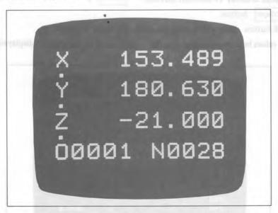
The current value in a programmed coordinate system set with G92, Automatic Coordinate System Setting, or by the following action (Reset) is displayed. For the T-axis, the presently selected tool number is displayed.
