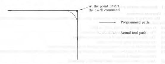
If the dwell command is inserted, the actual tool path matches the programmed path. The faster the feedrate and the larger the acceleration/deceleration time constant, the larger the error at the corner.
