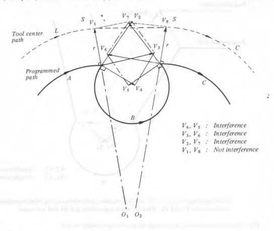
(Example 2) The tool moves linearly as follows: Tool path:  $V_1 \rightarrow V_2 \rightarrow V_7 \rightarrow V_8$
