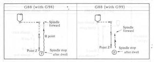
This command is equal to G87 (canned cycle I) except the spindle stops at the hole bottom after dwell.
