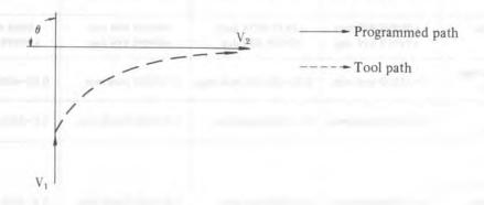
Fig. 4. 1 (a) Tool path in the corner
